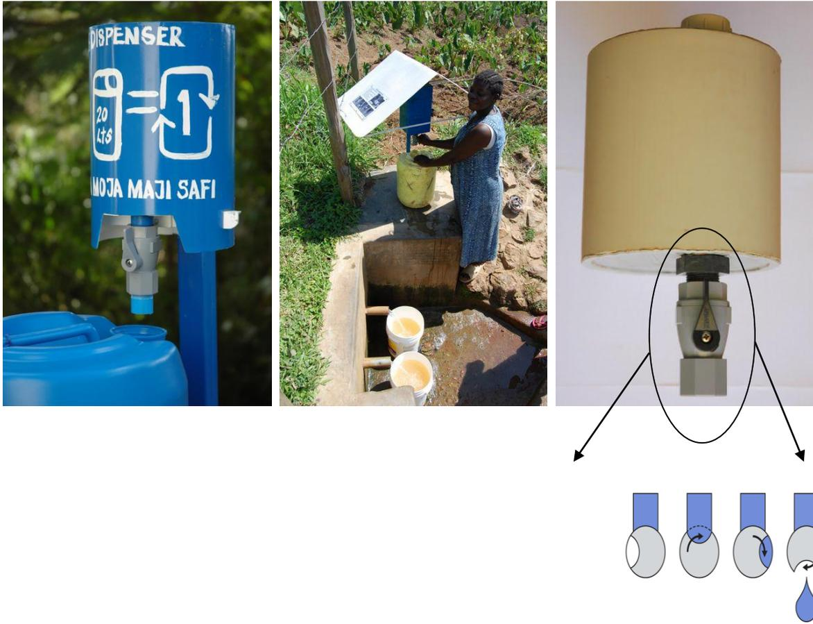
Notes: The dispenser is installed immediately next to a communal water source and delivers a 3 mL dose of dilute chlorine sufficient to treat 20 liters of water with each turn of the knob. Pictorial instructions are prominently displayed on the housing of the dispenser, which protects the chlorine storage tank inside from the elements. The dispenser tank holds three liters of dilute chlorine solution, enough to treat roughly a month supply for a community of a couple hundred people.
